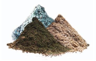
Final grain: approx. 150mm-200mm 4-fold fracture- and cutting-process in one shaft rotation
