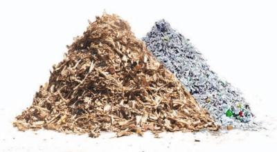
Final grain: approx. 200 mm - 500 mm Single fracture- and cutting-process in one shaft rotation
