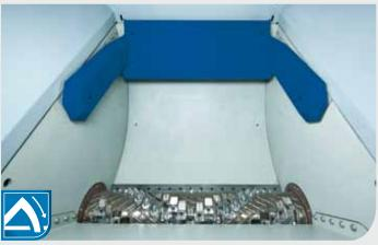
Rammer – internal hydraulic pusher system
