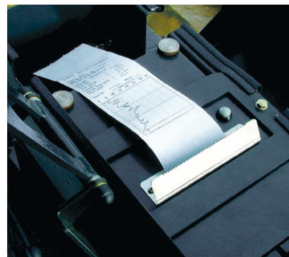
A data recorder documents compaction parameters (optional)
