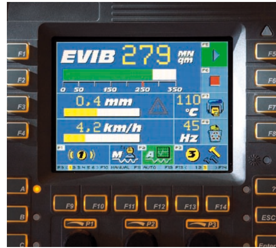
BOP (BOMAG Operational Panel) continually shows compaction progress
