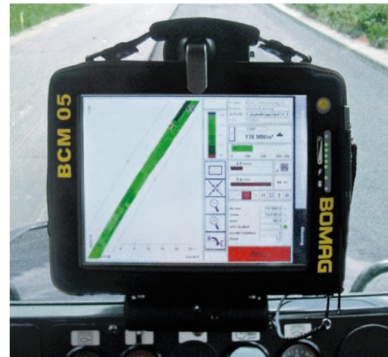
BCM (BOMAG Compaction Manager) for surface compaction control with GPS (optional)
