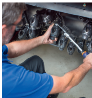
Fast and easy changes of tool holders on the milling drum.
